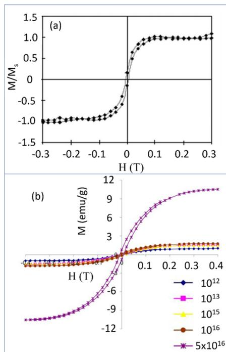
Fig. 9 (a) Magnetization ( $M$ ) versus applied field ( $H$ ) curves for the detonation NDs ( $d = 4-5$  nm) ( $M_s =$  saturation magnetization) with  $^{15}\text{N}$  dose at (a)  $5 \times 10^{14}$   $\text{cm}^{-2}$  and (b) various doses: enhanced magnetizations were observed with doses above  $5 \times 10^{16}$   $\text{cm}^{-2}$ .<sup>144</sup> Reproduced with permission from ref. 144 Copyright 2005 American Physical Society.
