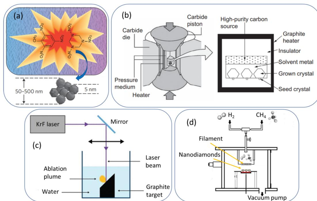
Fig. 1 (a) Detonation production of nanodiamonds,<sup>64</sup> (b) HPHT production of microdiamonds,<sup>78</sup> (c) laser ablation production of nanodiamonds,<sup>53</sup> and (d) CVD production of nanodiamonds.<sup>55</sup> Reproduced with permissions from ref. 64 Copyright 2012 Springer-Nature, ref. 78 Copyright 2016 Elsevier, and ref. 53 Copyright 2018 Springer.
