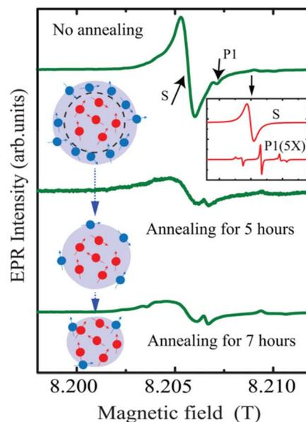
Fig. 8 EPR analysis of 50 nm NDs before and after air annealing for 5 and 7 h. The inset on the top right shows contributions of nitrogen impurity centers (labeled as P1) and surface spins (labeled as S) to the EPR spectra. The EPR spectra under the annealing process are shown below. The red dots in the drawing represent the P1 centers and the blue dots represent surface spins.<sup>143</sup> Reproduced with permission from ref. 143 Copyright 2020 American Institute of Physics.
