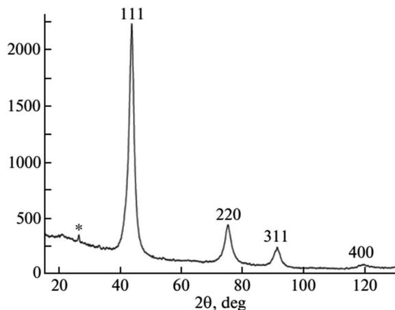
Fig. 4 XRD pattern of NDs produced by laser ablation ( $d = 3\text{--}4\text{ nm}$ ).<sup>114</sup> Reproduced with permission from ref. 114 Copyright 2013 Springer.
