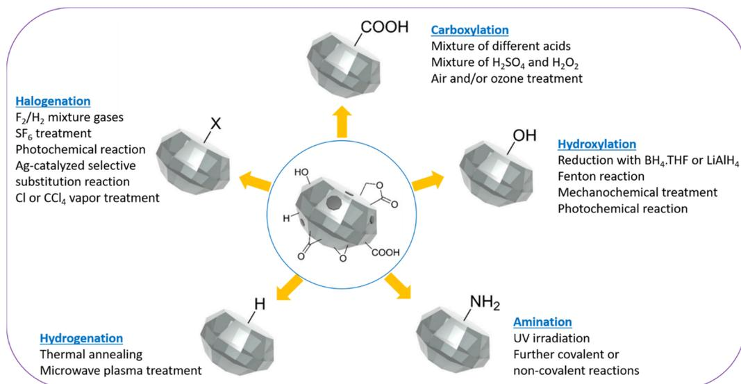
Fig. 2 Schematic representation of homogenization of ND surfaces *via* carboxylation, hydroxylation, hydrogenation, amination, and halogenation.<sup>87</sup>
