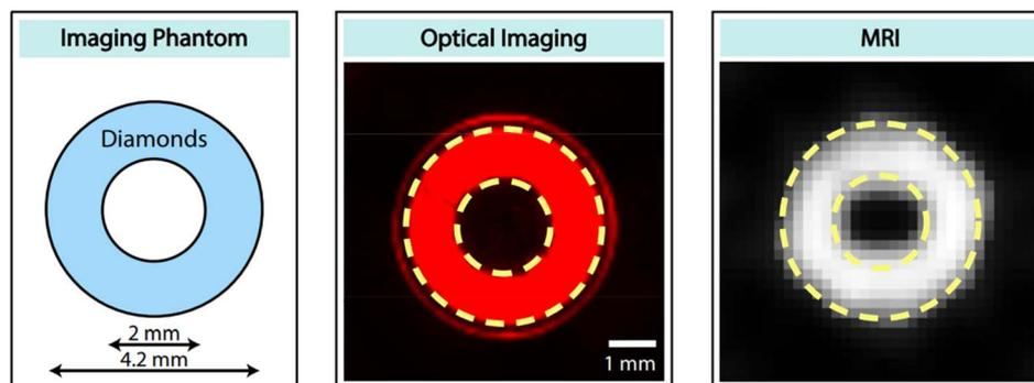
Fig. 19 Dual-modal optical and  $^{13}\text{C}$  MR imaging. (left) Ring-shaped phantom filled with 40 mg of 200  $\mu\text{m}$  diamonds. (middle) Fluorescence image with a 630 nm filter. (right)  $^{13}\text{C}$  MR image.<sup>176</sup> Reproduced with permission from ref. 176 Copyright 2021 National Academy of Sciences USA.
