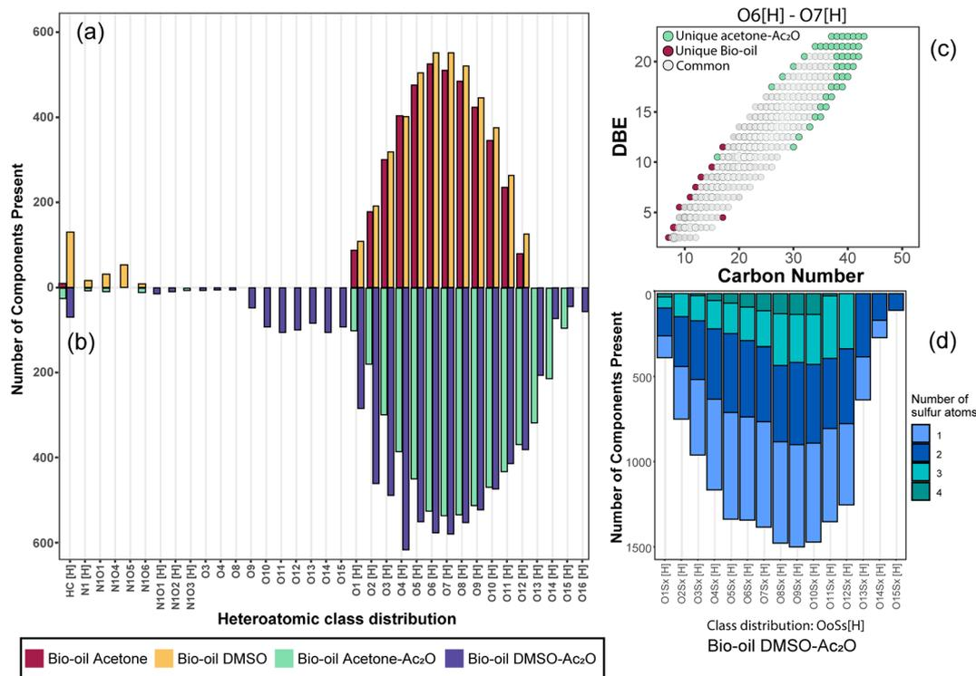
Fig. 2 Heteroatomic class distribution of the bio-oil: (a) before reaction (b) after reactions in the presence of acetic anhydride. (c) DBE plot for classes  $O_6[H]$  and  $O_7[H]$  before and after derivatisation, common species represent overlapping molecular compositions, and (d) class distribution of the sulfur–oxygen containing species, detected only in the sample bio-oil  $DMSO-Ac_2O$ .
