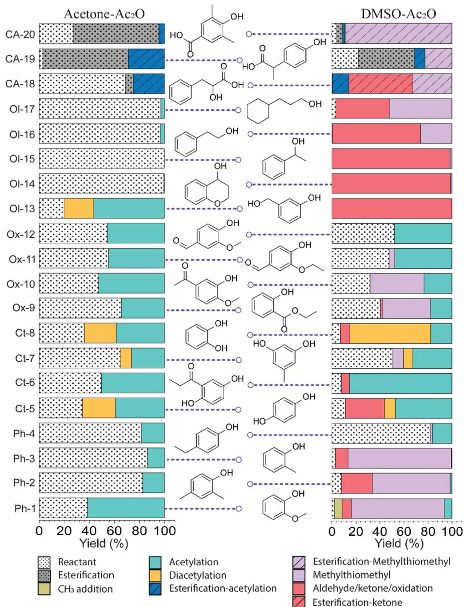
Fig. 1 Reaction yields observed on lignin-representative standard molecules in mixtures of acetone-Ac<sub>2</sub>O and DMSO-Ac<sub>2</sub>O.
