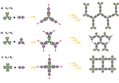
Scheme 4 Schematic of conventional step polymerization to yield polymer networks using multifunctional (a) A<sub>3</sub> + B<sub>2</sub>, (b) A<sub>3</sub> + B<sub>3</sub>, and (c) A<sub>4</sub> + B<sub>2</sub> monomers.
