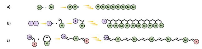
Scheme 6 Schematic diagrams of (a) chain polymerization (generic mechanism), (b) vinyl polymerization, and (c) ROMP.
