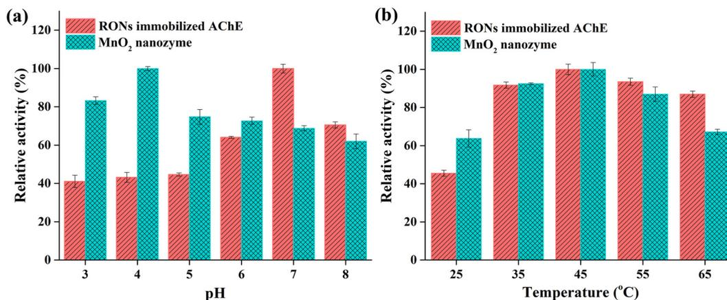
Fig. 7 (a) pH stability and (b) thermal stability of RONS immobilized AChE and MnO<sub>2</sub> nanozyme.
