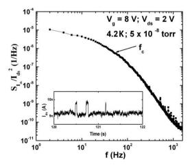
Fig. 5 Lorentzian noise power spectrum for a ZnO NW exhibiting random telegraph noise, RTN, at a temperature of 4.2 K. The corner frequency  $f_c$  is ~18 Hz. The inset plots current vs. time. Reproduced from ref. 62 with permission. Copyright 2007 American Institute of Physics.
