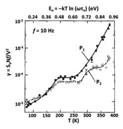
Fig. 3 Normalized noise magnitude vs. temperature for two Pt NWs. The energy  $E_0$  that corresponds to the temperature T via eqn (7) is shown on the upper x-axis, assuming  $\tau_0 \approx 10^{-14}$  Hz. Adapted from ref. 96 with permission. Copyright 1987 American Institute of Physics.
