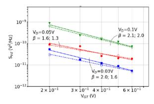
Fig. 28 Gate-voltage dependence of  $S_{V_d}$  at  $V_{\rm DS}=30$  mV, 50 mV, and 100 mV for as-processed (closed symbols, solid lines) and irradiated (open symbols, dashed lines) GAA NW nFETs. The device was irradiated to 1 Mrad(SiO<sub>2</sub>) with 10 keV X-rays at  $V_{\rm GS}=0.5$  V. Reproduced from ref. 74 with permission. Copyright 2021 Institute of Electrical and Electronics Engineers.
