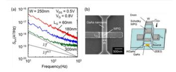
Fig. 19 (a) Current noise power-spectral densities of Schottky wrapgate (WPG) GaAs/AlGaAs NW transistors with W = 250 nm and varying L. (b) Top view and schematic cross-section. Adapted from ref. 64 with permission. Copyright 2011 Institute of Physics.
