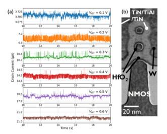
Fig. 25 Gate-to-threshold voltage dependence of  $I_{\rm DS}$  at 295 K for a GAA NW nFET with  $L\approx 25$  nm, 8 nm diameter, and 1.8 nm HfO<sub>2</sub>/1 nm gate dielectric; a transmission-electron-microscope image of the structure is shown in (b).  $V_{\rm DS}=50$  mV;  $V_{\rm GT}\equiv V_{\rm GS}-V_{\rm TH}.$  Note that each value of  $V_{\rm GT}$  has a different y-axis scale. Adapted from ref. 74 with permission. Copyright 2021 Institute of Electrical and Electronics Engineers.
