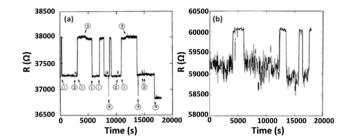
Fig. 14 (a) Resistance vs. time at T=70 mK for an  $\sim 8$  nm thick Bi film with L=10  $\mu$ m and W=4  $\mu$ m. Numbers denote different fluctuators. (b) Resistance vs. time at 250 mK for a 1 nm thick Pt film with L=7  $\mu$ m and W=5  $\mu$ m. Adapted from ref. 54 with permission. Copyright 1987 Institute of Physics.
