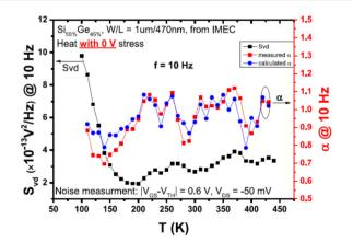
Fig. 6 Noise magnitude (left y-axis) and measured and predicted values of  $\alpha = -\partial \ln S_V/\partial \ln f$  vs. temperature (right y-axis) for a SiGe pMOSFET with  $SiO_2/HfO_2$  gate dielectric. Predicted  $\alpha$  values are derived from the  $S_{V_a}$  vs. T curve measured before bias-temperature stress, using eqn (5) of the text. Reproduced from ref. 133 with permission. Copyright 2016 Institute of Electrical and Electronics Engineers.
