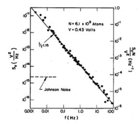
Fig. 1 Excess voltage-noise power spectral density  $S_V$  as a function of frequency f for a Pt nanowire (NW) fabricated via substrate step lithography. The Johnson (thermal) noise background has been subtracted. The size and voltage normalized noise,  $S_V N/V_s^2$  is shown on the right-h and y-axis, with  $N = N_A$ . Reproduced from ref. 51 with permission. Copyright 1983 The American Physical Society.
