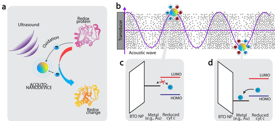
**Fig. 3** Protein oxidation by acousto-nanodevice driven under external acoustics. (a) principle of acousto-nanodevice-driven protein redox (b) The work function of the surface metal of the acousto-nanodevice oscillates under incoming acoustic waves, (c–d) a unidirectional electron transfer from protein to acousto-nanodevice is achieved because of the band alignment between the surface metal and the HOMO/LUMO levels of the protein redox center.
