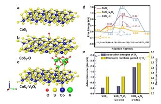
Fig. 5 (a-c) Crystal structures of  $CoS_2$ ,  $CoS_2$ -O and  $CoS_2$ - $V_2O_5$ , (d) comparison of standard Gibbs free energies at the rate determining step of CoS<sub>2</sub>, CoS<sub>2</sub>-O and CoS<sub>2</sub>-V<sub>2</sub>O<sub>5</sub> during the HER process, and (e) the adsorption energies of O2 molecules at metal sites (Co sites and V sites) and the electronic numbers gained by O2 molecules.
