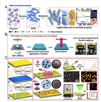
(A) Schematic diagram of the preparation of multifunctional nanoparticles; (B) schematic diagram of spin-coating for the preparation of PUF security labels. Reproduced with permission from ref. 66. Copyright 2021 Elsevier. (C) Schematic diagram of adsorbed nanoparticles after the preparation of random micro-regions using dry instability. Reproduced with permission from ref. 68. Copyright 2021 American Chemical Society.
