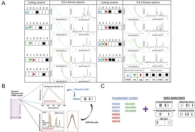
Fig. 8 (A) Raman-fluorescence combined encoding for security labels; Raman-absorption combined encoding for security labels. Reproduced with permission from ref. 60. Copyright 2016 American Chemical Society. (B) Schematic diagram of the encoding source; (C) double layer encoding – plasmonic encoding and Raman encoding. Reproduced with permission from ref. 61. Copyright 2015 John Wiley & Sons, Inc.
