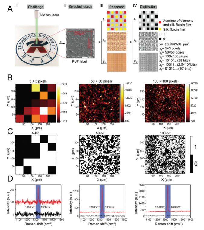
Fig. 11 (A) Schematic diagram of encoding the PUF label; (B) Raman imaging of the PUF label; (C) the binary-encoded map corresponding to the image; (D) corresponding binary Raman spectrogram. Reproduced with permission from ref. 67. Copyright 2021 John Wiley & Sons, Inc.
