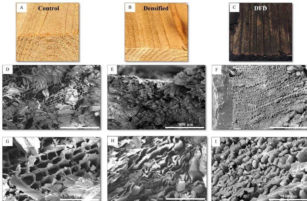
**Fig. 3** Images of actual sample (A) control, (B) delignified densified, and (C) DFD (delignified and *in situ* functionalized densified). SEM images of cross-sectional morphology (D), (E) and (F) show the magnified image (HFW\*: 1 mm) for the original, delignified densified, and the DFD samples respectively; SEM images (G), (H) and (I) show the magnified image (HFW\*: 250  $\mu\text{m}$ ) for the original, delignified densified, and the DFD samples respectively. \*Horizontal field width.
