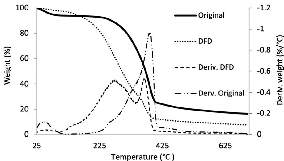
**Fig. 4** Thermogravimetric/derivative thermogravimetric (TG/DTG) curves of original wood (untreated), *in situ* functionalized densified wood (DFD); deriv: derivative TG curve. The derivative curve for DFD sample shows an extra peak (100–300  $^{\circ}\text{C}$ ) corresponding to the degradation of polymerized LAO which was not visible for the original wood.
