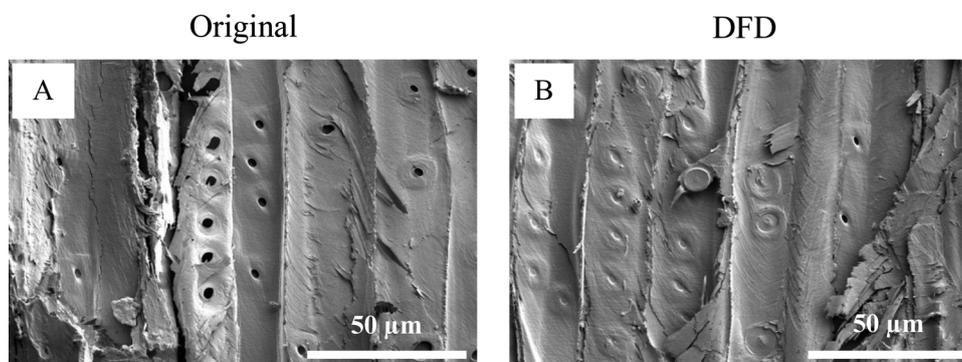
**Fig. 6** SEM images of the original wood and DFD surface showing the open pores (pits) 'A' and closed/clogged pits 'B'. Open pores allow the transfer of minerals and water to the adjacent cell wall. Closing them by blocking or filling up with polymers improves the water repellency property of wood.
