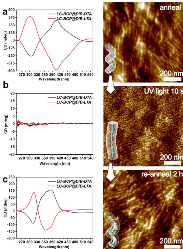
**Fig. 6** CD spectra and AFM image of LC-BCP@DiB-LTA film before and after (b) UV irradiation (10 s, 365 nm, 150 mW cm<sup>-2</sup>), and the recovered helical structure after re-annealing for 2 h (c).
