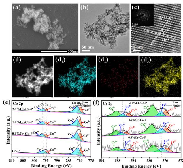
Fig. 4 SEM and TEM images of 1.2% Cr-Co-P (a and b). (c and inset c) the corresponding high-resolution images and SAED patterns. (d–d<sub>3</sub>) Corresponding elemental mappings of 1.2% Cr-Co-P with Co (d<sub>1</sub>), Cr (d<sub>2</sub>) and O (d<sub>3</sub>). (e) Co 2p and (f) Cr 1s XPS spectra of M% Cr-Co-P.
