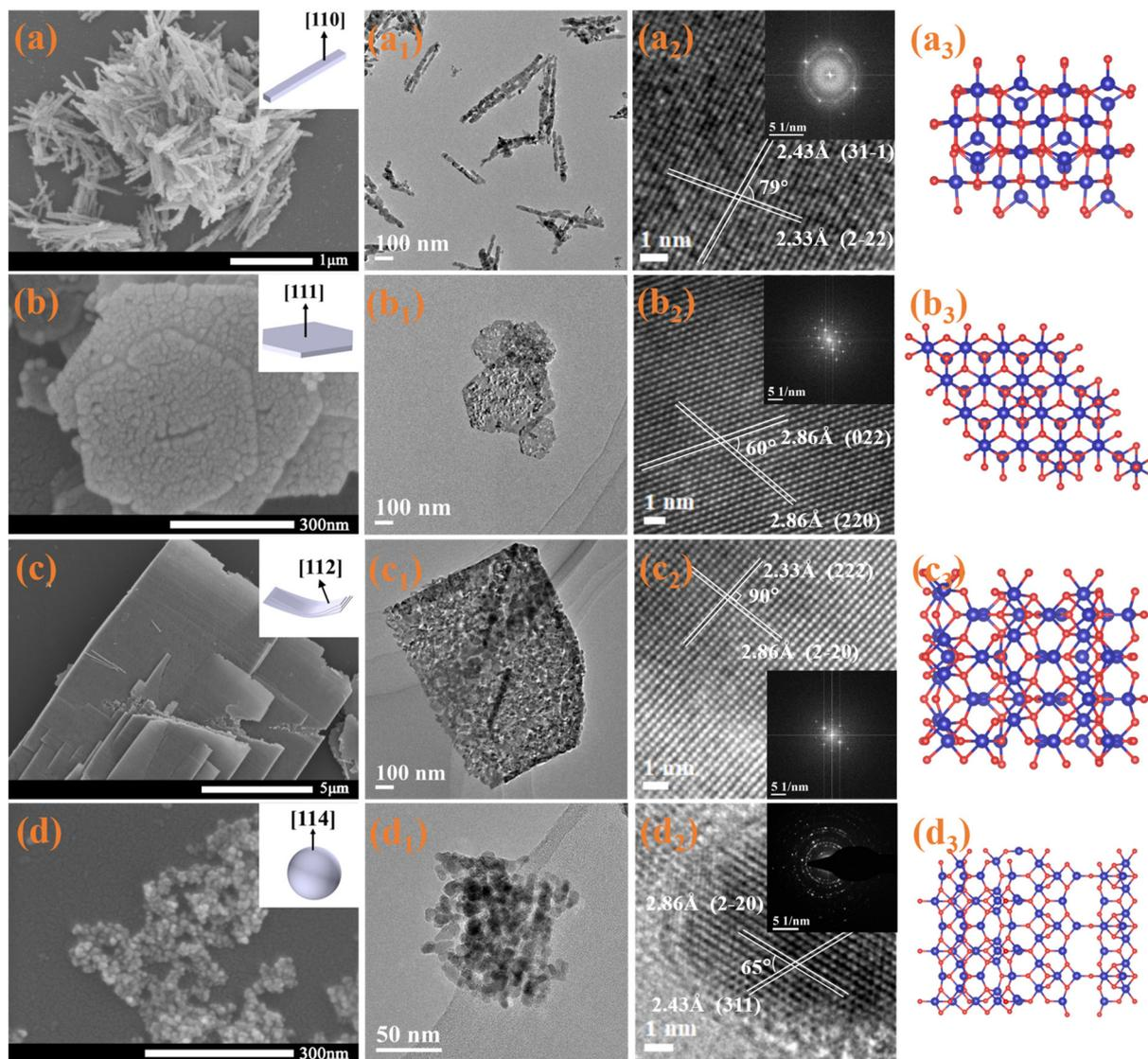
**Fig. 1** SEM and TEM images of Co-R (a and a<sub>1</sub>), Co-H (b and b<sub>1</sub>), Co-L (c and c<sub>1</sub>) and Co-P (d and d<sub>1</sub>) (insets show the corresponding 3D models of Co<sub>3</sub>O<sub>4</sub>). a<sub>2</sub>, b<sub>2</sub>, c<sub>2</sub> and d<sub>2</sub> show the corresponding high-resolution images and SAED patterns. Surface atomic structure models of (110), (111), (112) and (114) facets (a<sub>3</sub>, b<sub>3</sub>, c<sub>3</sub> and d<sub>3</sub>).
