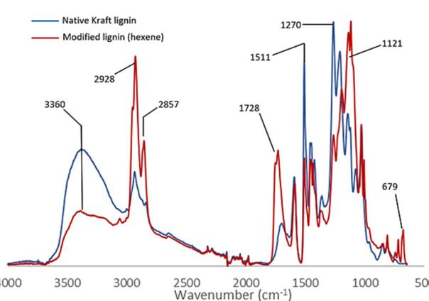
**Fig. 2** Comparison of IR spectra of technical (blue) and modified kraft lignin (red).
