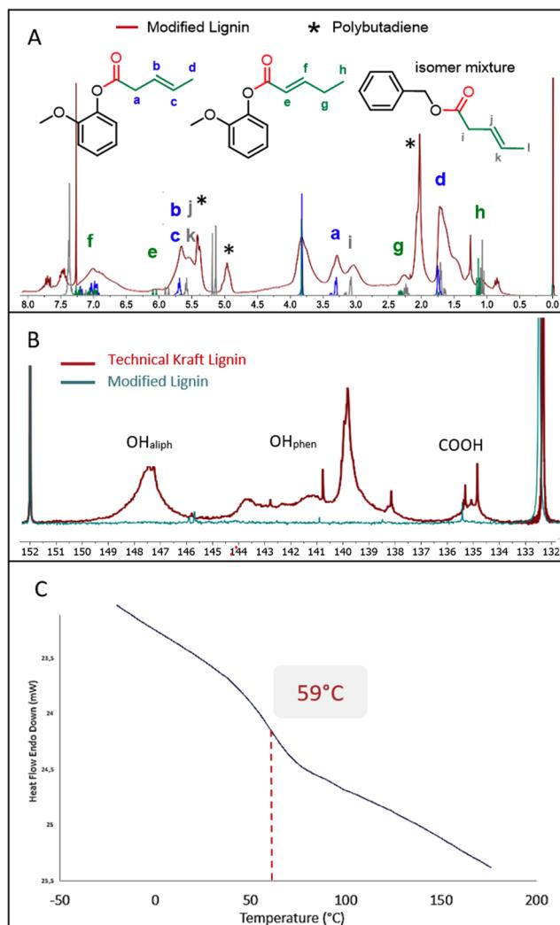
**Fig. 5** <sup>1</sup>H NMR (A), <sup>31</sup>P NMR with intensities calibrated on the internal standard (B) and DSC (C) analysis of the product of hydroesterification of butadiene with Kraft lignin (Table 5, entry 5).
