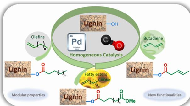
**Scheme 1** Overall scheme for Pd-catalyzed hydroesterification on lignin.
