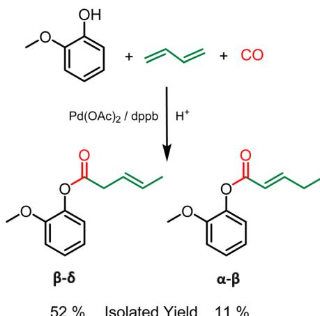
**Scheme 3** Hydroesterification of butadiene with guaiacol – Reaction conditions: Guaiacol 9 mmol, benzoic acid 0.3 eq., butadiene 7 eq.,  $\text{Pd}(\text{OAc})_2$  1 mol%, dppb 6 eq./Pd, 120 °C, 24 h, 25 bar CO, THF.
