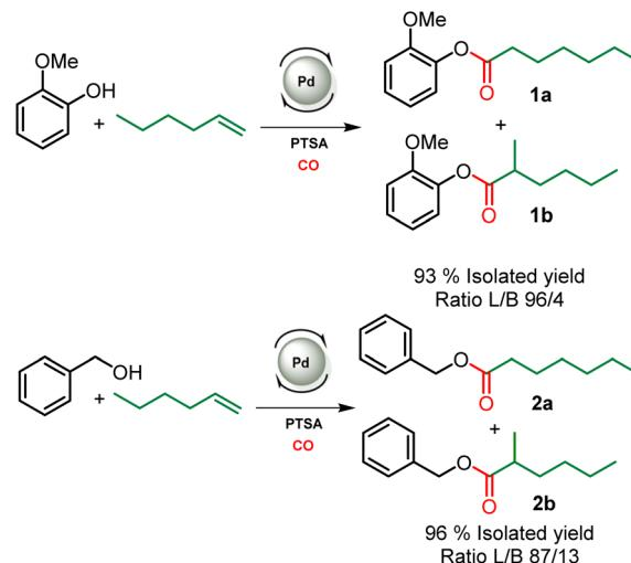
**Scheme 2** Hydroesterification of 1-hexene with guaiacol (top) and benzyl alcohol (bottom). Reaction conditions: [Pd]: Pd(OAc)<sub>2</sub>/PPh<sub>3</sub> – 120 °C, 22 h, 30 bar CO, THF. L/B ratio determined in <sup>1</sup>H NMR, see Fig. S11.†
