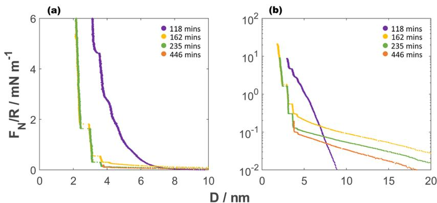
**Fig. 10** Normalised force profiles as a function of surface separation for 80 vol% EAN. (a) Surface separation less than 10 nm showing 4 different profiles measured at different time after liquid injection: purple at 118 min, yellow at 162 min, green at 235 min and orange at 446 min. (b) Log–linear scale of the same profiles as (a) with surface separation displayed up to 20 nm.
