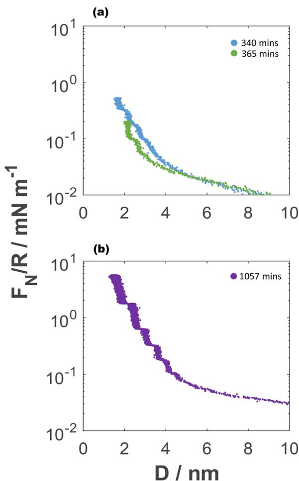
Fig. 9 Time evolution of the normalised force between mica sheets as a function of separation,  $D$ , across 90 vol% EAN at the same spot. (a) Measured at 340 min and 365 min after liquid injection. (b) Measured at 1057 min after liquid injection.
