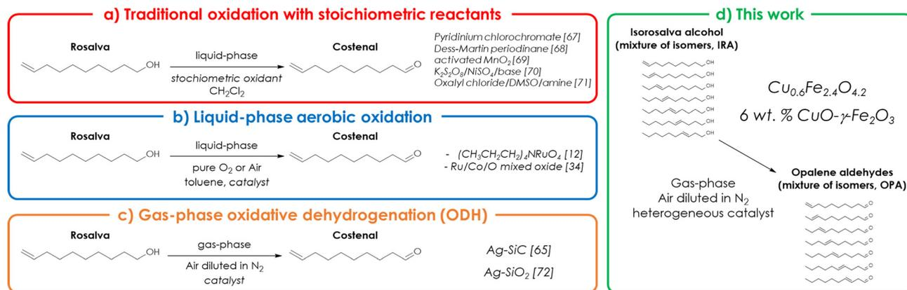
**Scheme 1** Comparison between a) oxidation of Rosalva to Costenal with traditional stoichiometric oxidants, b) aerobic oxidation of Rosalva with air/O<sub>2</sub> in the liquid-phase, c) oxidative dehydrogenation (ODH) of Rosalva in the gas-phase and d) oxidative dehydrogenation (ODH) of an Isorosvalva mixture of isomers in the gas-phase.
