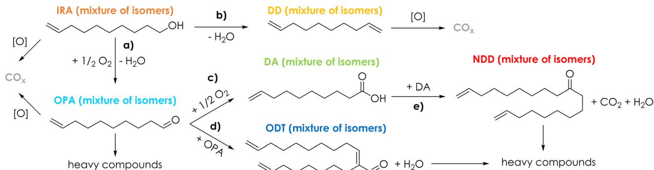
**Scheme 3** Proposed complete reaction scheme: a) ODH of IRA towards OPA; b) parallel parasitic dehydration of IRA towards DD; c) overoxidation of OPA towards DA; d) aldol condensation of OPA to ODT; e) ketonization of DA to NDD; other reactions include the formation of heavy compounds on the catalyst surface and the total oxidation to  $\text{CO}_x$ .
