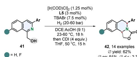
**Scheme 9** *trans*-Selective directed enantioselective hydrogenation of 1,3-disubstituted isoquinolines with subsequent formation of an oxazolidine-2-one by Stoltz and co-workers.<sup>63</sup>
