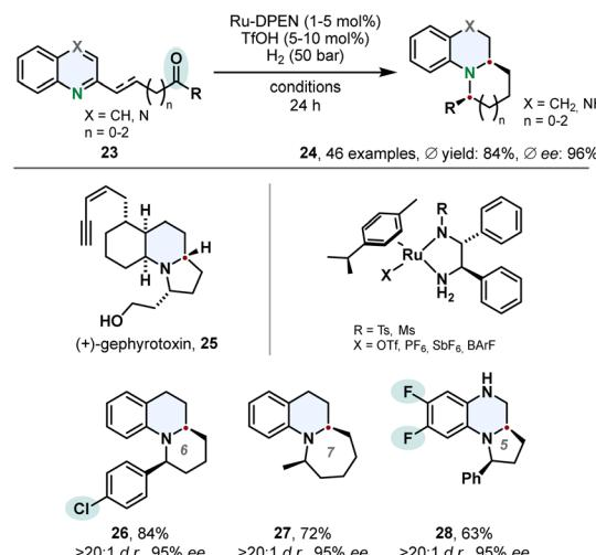
Scheme 6 Cascade hydrogenation-condensation strategy for the synthesis of chiral indolizidines and quinolizidines involving an enantioselective hydrogenation published by Fan and co-workers.<sup>57</sup>
