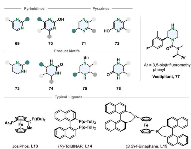
Fig. 8 Top: Overview of pyrimidines and pyrazines successfully employed in an enantioselective hydrogenation reaction.<sup>93–97</sup> Middle: Corresponding product motifs after hydrogenation. Bottom: Examples for successfully used ligands in these hydrogenation reactions.
