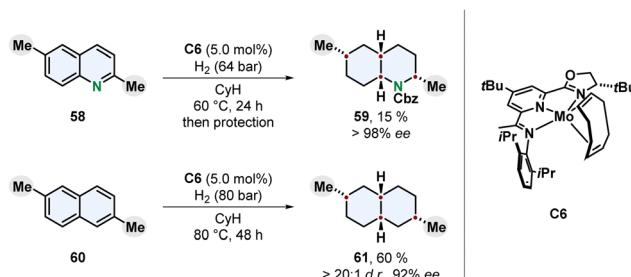
**Scheme 12** Molybdenum catalysed enantioselective full hydrogenation of quinolines and naphthalenes to the corresponding decahydroquinolines and decalin by Chirik and co-workers.<sup>79</sup>
