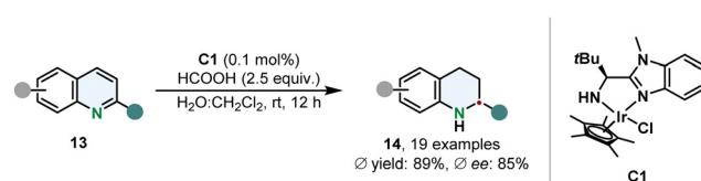
Scheme 3 Transfer hydrogenation of 2-substituted quinolines with a water-soluble chiral iridium complex by Sun and co-workers.<sup>53</sup>
