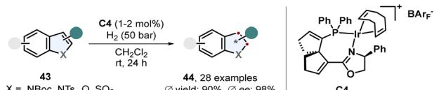
Scheme 10 Iridium catalysed enantioselective hydrogenation of 2- and 3-substituted indoles and benzofurans by Han, Ding and co-workers.<sup>64</sup>
