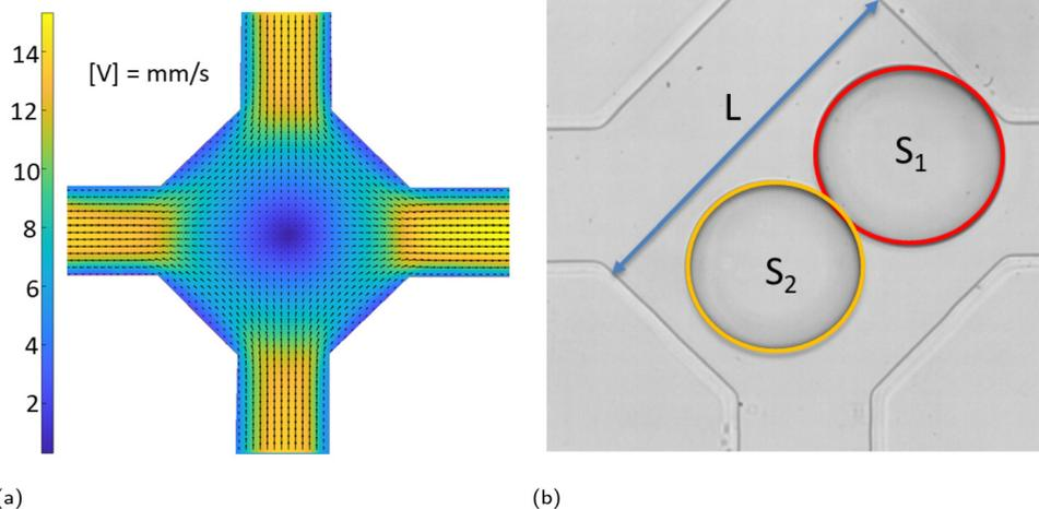
Fig. 1 Drop coalescence experiments in a microfluidic device.
