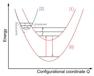
Schematic overview of the different processes determining the performance of a luminescent crossover thermometer such as Sm<sup>2+</sup> Curvy arrows indicate (multi-)phonon absorption transitions. Note that the excited state |2| has been depicted at lower configurational coordinates to match the theoretical and experimental findings for low excited  $4f^{n-1}5d^1$  states of lanthanoid ions (see also text)
