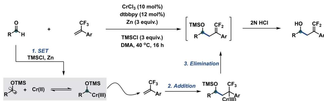
C. This Work: Catalytic Defluorinative Ketyl-Olefin Coupling by *Halogen-Atom Transfer* (XAT) - Unknown
