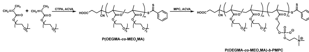
Scheme 1 Synthesis of P(OEGMA-*co*-MEO<sub>2</sub>MA)-*b*-PMPC.
