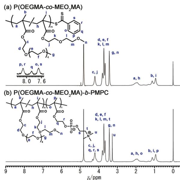
Fig. 2 <sup>1</sup>H NMR spectra of (a) P(OEGMA-*co*-MEO<sub>2</sub>MA) and (b) P(OEGMA-*co*-MEO<sub>2</sub>MA)-*b*-PMPC.
