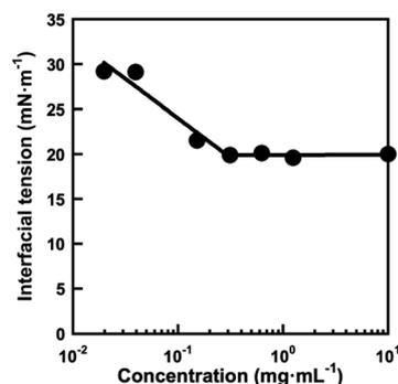
**Fig. 4** Effect of P(OEGMA-co-MEO<sub>2</sub>MA)-*b*-PMPC concentration on the interfacial tension of a water–chloroform interface at 25 °C. The interfacial tension was measured using the pendant drop technique with a contact angle meter.
