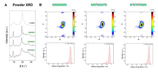
Fig. 7 (A) Powder XRD profiles of 6F-chitin compared to  $\alpha$ -chitin profile (dotted line). (B) Ramachandran plots for all glycosidic linkages combined (top) and radius of gyration plots (bottom) extracted from the MD simulations.
