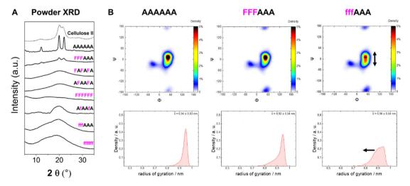
Fig. 5 (A) Powder XRD profiles of 3F- and 6F-cellulose compared to cellulose II profile (dotted line). (B) Ramachandran plots for all glycosidic lin-kages combined (top) and radius of gyration plots (bottom) extracted from the MD simulations. The dihedral angles are defined as  $\Phi$  = H1C1O4C4 and  $\Psi$  = C1O4C4H4 (further details are reported in Fig. S3 in the ESI†).
