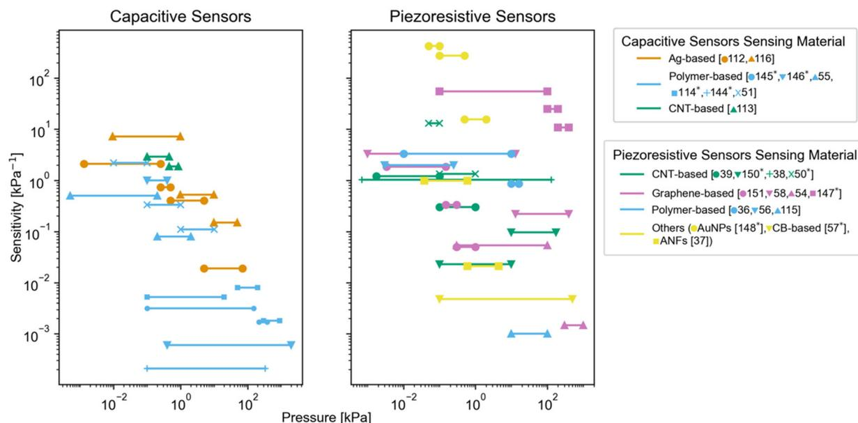
**Fig. 6** Sensitivity as a function of the pressure range of recently reported printed flexible pressure sensors grouped by the sensing material and sensor type (capacitive and piezoresistive). \* These works did not report a lower detection limit for their sensor; therefore, a value of 100 Pa was assumed to use a logarithmic scale on the x-axis.
