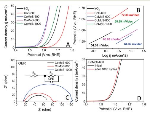
Fig. 7 (A) OER polarization curves and (B) corresponding Tafel plots of the benchmark IrO<sub>2</sub>, CoS-600, CoMoS-600, CoMoS-800 and CoMoS-1000. (C) EIS of CoMoS-600, CoMoS-800 and CoMoS-1000. (D) Polarization curves of CoMoS-600 before and after 1000 CV cycles. All polarization curves are iR corrected
