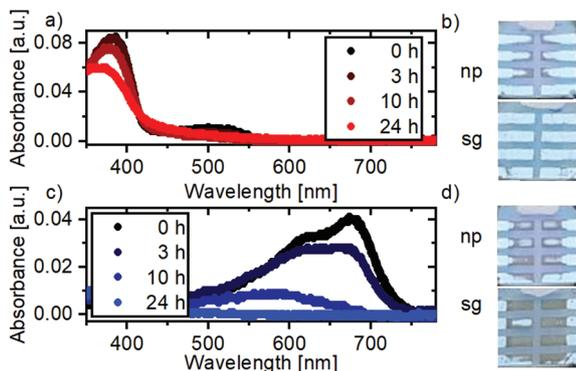
**Fig. 6** Dry air and sunlight degradation of the HTL. (a) Absorption changes of a PTAA:C<sub>60</sub>F<sub>48</sub> film. (b) Picture of the electrode of a device using PTAA:C<sub>60</sub>F<sub>48</sub> after 42 h of degradation with either ZnO nano-particle or sol-gel as ETL. (c) Absorption changes in PTB7. (d) Pictures of solar cell electrodes employing PTB7 as HTL and either nano-particle or sol-gel ZnO as ETL.
