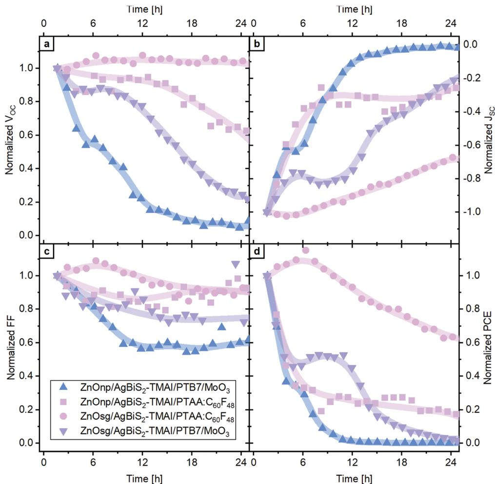
**Fig. 2** Photovoltaic evolution in dry air with continuous 1 sun illumination of AgBiS<sub>2</sub> NC solar cells with different extraction layers. The photovoltaic parameters, (a)  $V_{OC}$ , (b)  $J_{SC}$ , (c) FF and (d) PCE, were averaged from several devices and normalized to their initial value. A guide for the eye in form of a line is added.
