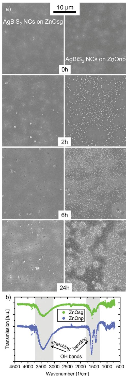
**Fig. 7** (a) SEM pictures of a AgBiS<sub>2</sub>-TMAI NC film on a ITO/ZnOsg (left column) or np (right column) layer during degradation in dry air and sunlight for different time steps. (b) FTIR measurements of a pristine ZnOsg and np film. The OH vibration bands are indicated and the data is offset to each other for better visibility.
