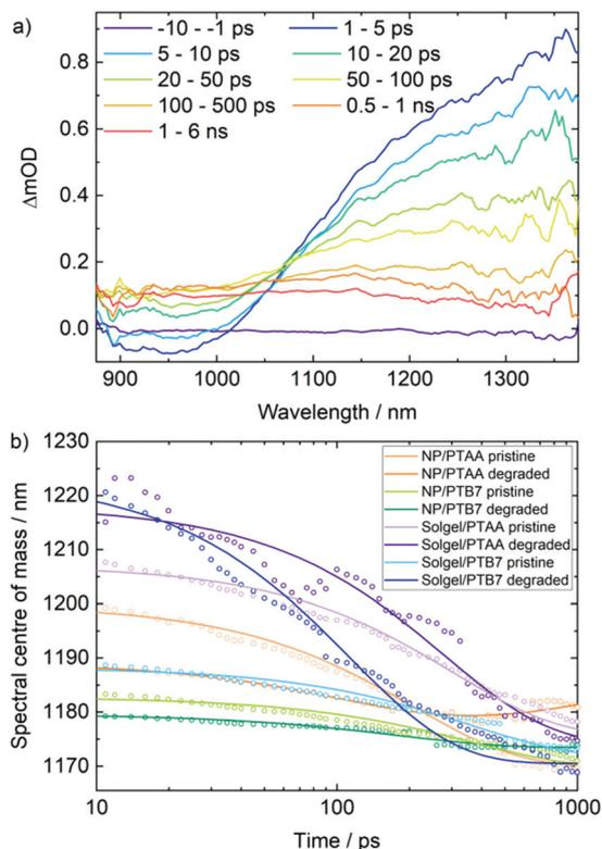
Fig. 4 (a) TA spectrum for degraded nanoparticle ZnO/AgBiS<sub>2</sub>-TMAI/PTB7 device following a 700 nm pump excitation. (b) Centre of mass of PIA signal as a function of time for each device configuration.
