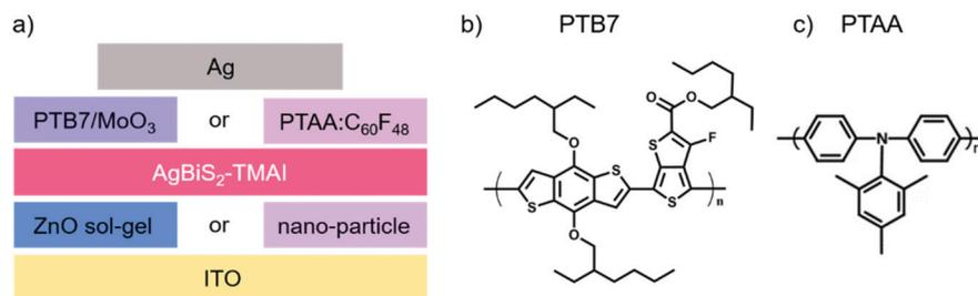
**Fig. 1** Structure of devices and materials. (a) Architecture of the studied solar cells. The HTL consists either of PTB7/MoO<sub>3</sub> or PTAA:C<sub>60</sub>F<sub>48</sub> and the molecular structure is shown in (b) and (c) for the polymers, respectively. The ETL was made from ZnO but either in a sol–gel thin film or as nano-particles, resulting in overall four combinations which were examined.
