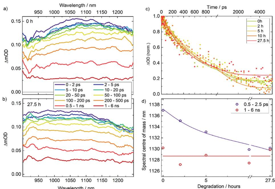
**Fig. 3** Transient absorption spectra for neat  $\text{AgBiS}_2$  films after (a) 0 h and (b) 27.5 h degradation following a 700 nm excitation. (c) Evolution in time of the normalised TA PIA signal for all films. (d) Centre of mass of PIA signal as a function of degradation time for early and late pump–probe time delays.
