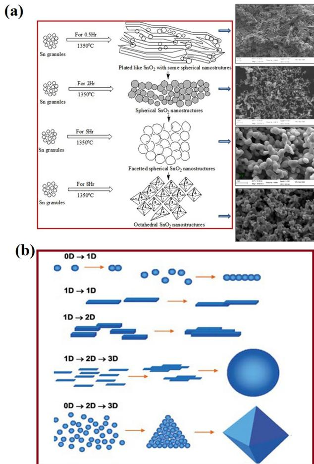
Fig. 7 (a) Schematic of the SnO<sub>2</sub> structural growth phenomena and morphological transformation with increasing evaporation time during thermal evaporation at 1350 °C. Reprinted with permission from ref. 152. Copyright 2014 Elsevier. (b) Various organizing schemes for the self-construction of nanostructures by oriented attachment. Reprinted with permission from ref. 151. Copyright 2004 John Wiley and Sons.
