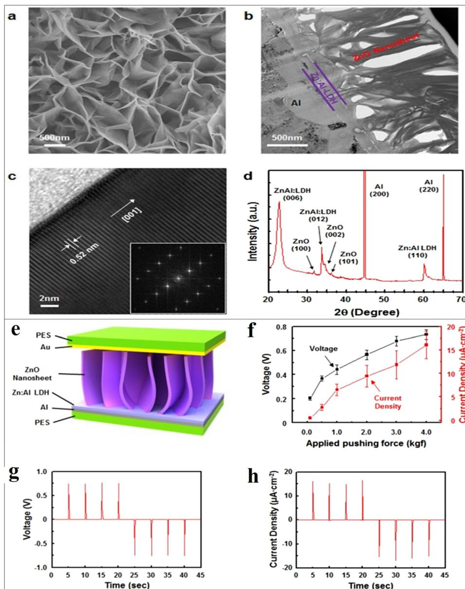
**Fig. 23** (a) Morphology of the ZnO nanosheets network structure grown on an Al substrate. (b) TEM (cross-sectional image) of the ZnO nanosheets network. (c) HR TEM image and corresponding FFT pattern (inset). (d) Synchrotron XRD pattern of the ZnO nanosheets (e–g). Schematic image and output voltage from the ZnO nanosheet-based nanogenerator. (h) Measured current density of the ZnO nanosheet-based nanogenerator. Reprinted with permission from ref. 277. Copyright 2013 Springer Nature.
