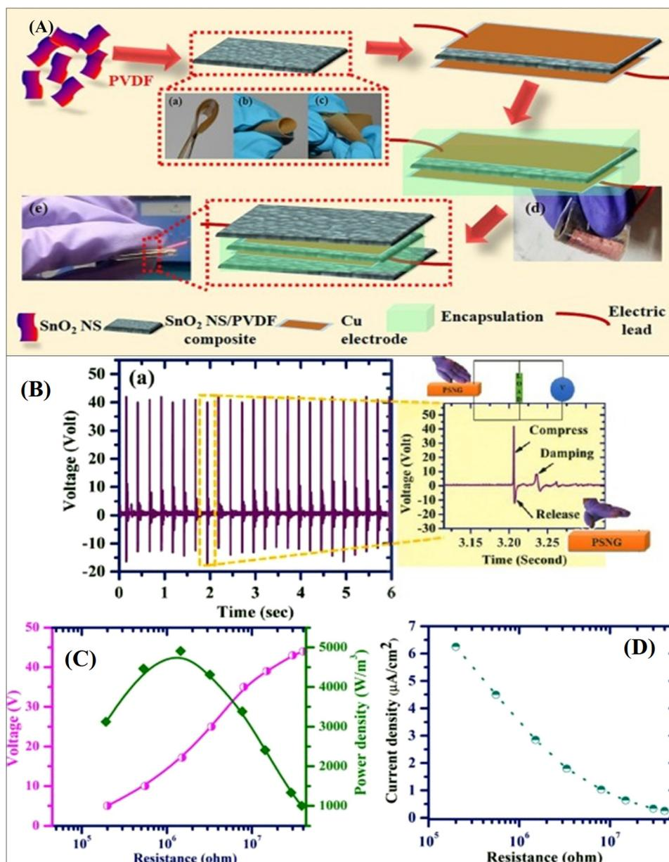
Fig. 24 (A) Schematic image of the fabrication procedure of the SnO<sub>2</sub>NS/PVDF-based nanogenerator (a–e). (B) Output voltage produced from the SnO<sub>2</sub>NS/PVDF nanogenerator. (C) Variation of the output voltage and (D) power density with load resistance. Reprinted with permission from ref. 282. Copyright 2019 Elsevier.
