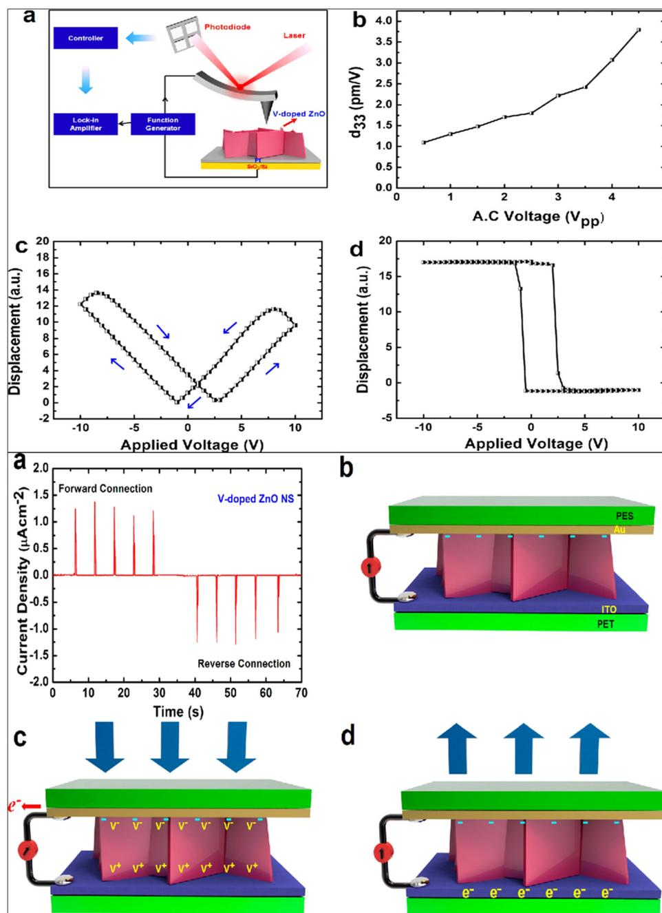
Fig. 21 (a) Experimental diagram of the piezoelectric response ( $d_{33}$ ) measurement through the PFM setup. (b–d) Butterfly curve and phase-voltage hysteresis curve. (e) The current density obtained from the V-doped ZnO nanosheets showing DC-type charge generation. Mechanism of charge generation of the V-doped ZnO device. Reprinted with permission from ref. 272. Copyright 2013 American Chemical Society.
