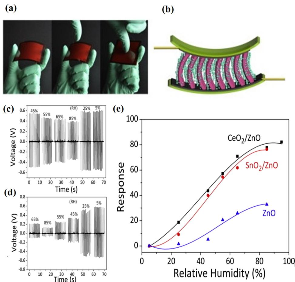
Fig. 25 (a and b) The original picture of the ZnO/SnO<sub>2</sub>-based flexible device under compressive deformation through human fingers. (c and d) Piezoelectric output voltage signal measured under different relative humidity conditions. (e) Response of the device under different relative humidity conditions. Reprinted with permission from ref. 284. Copyright 2014 Elsevier.
