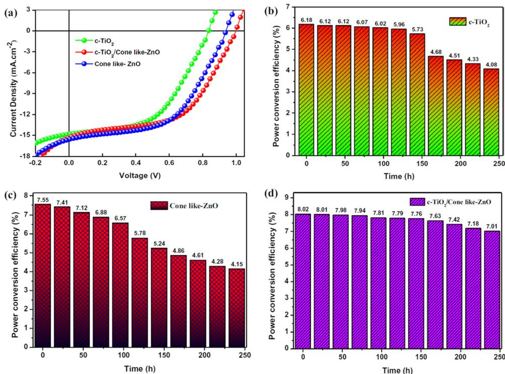
Fig. 8 Use of cone-like ZnO improves the perovskite solar cell performance. (a) Better  $J$ - $V$  characteristics of upon addition of the cone-like ZnO as a part of ETL. (b-d) PCE over time for the single layer c-TiO<sub>2</sub>, cone-like ZnO and bilayer of c-TiO<sub>2</sub> with cone like ZnO as ETL. Reprinted with permission from ref. 180. Copyright 2021 Springer Nature.
