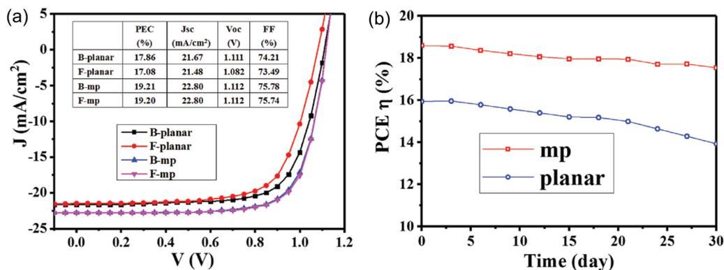
Fig. 11 (a)  $J$ - $V$  graphs obtained of the planar  $\text{SnO}_2$  and mp  $\text{SnO}_2$  PSCs from under backward and forward voltage scanning. (b) PCEs of the planar  $\text{SnO}_2$  and mp  $\text{SnO}_2$  PSCs monitored every 3 d; the measurement was performed under AM 1.5G with input solar power  $P_{\text{in}}$  of  $100 \text{ mW cm}^{-2}$ . Reprinted with permission from ref. 224. Copyright 2018 John Wiley and Sons.
