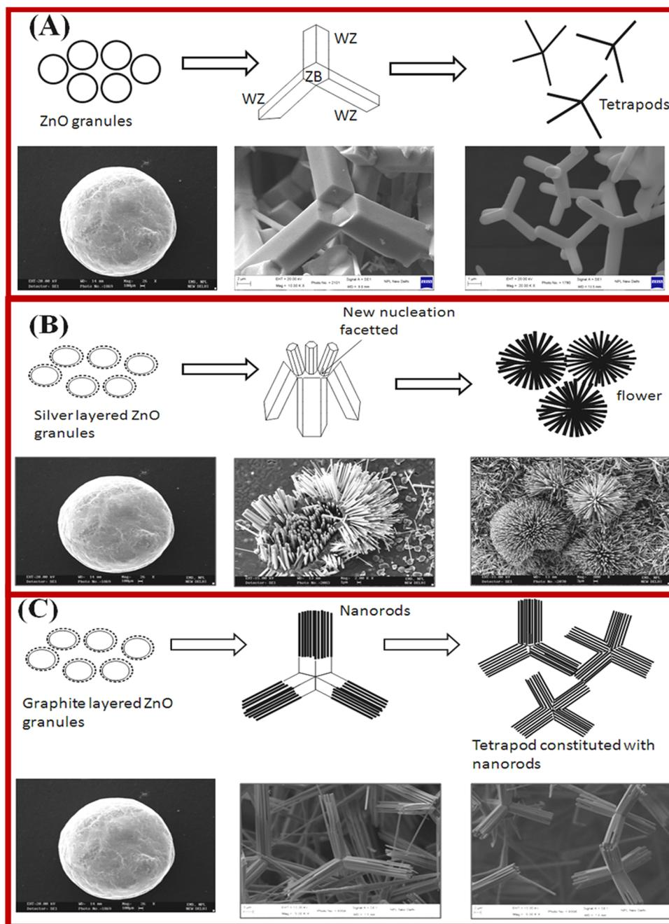
Fig. 4 Presentation of ZnO tetrapod structures nucleation and growth kinetics, and microstructural transformation with Ag and graphite doping. (a–c) ZnO, Ag-doped ZnO and Gr-doped ZnO. Reprinted with permission from ref. 116. Copyright 2013 Elsevier.
