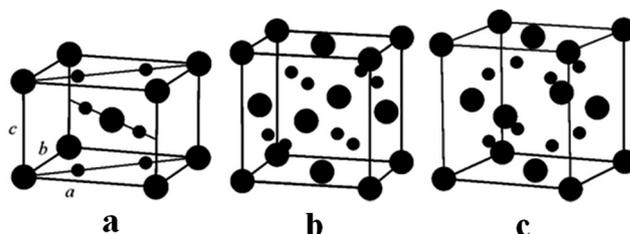
Fig. 5 Crystal structures of the SnO<sub>2</sub> nanostructures: (a) tetragonal rutile, (b) cubic pyrite, (c) cubic fluorite. Large and small circles represent the Sn and O atoms, respectively. Reprinted with permission from ref. 132. Copyright 2012 Springer Nature.
