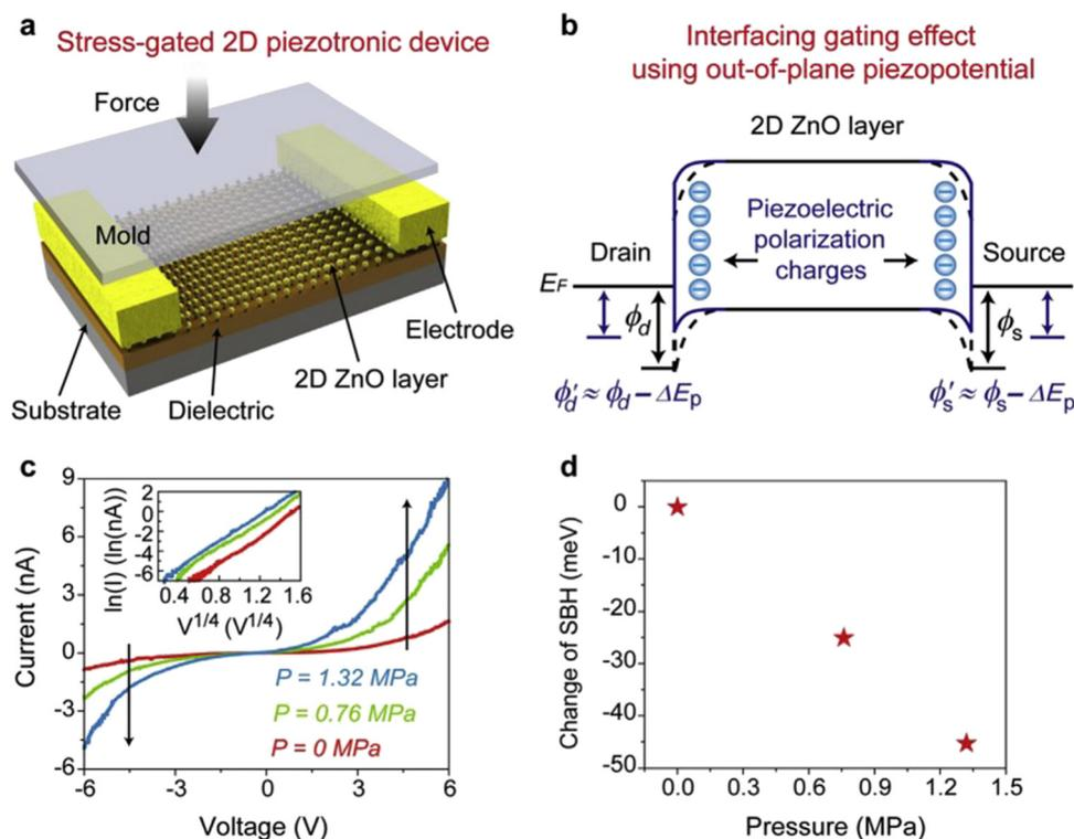
Fig. 27 (a and b) Schematic device diagram of the stress-gated 2D layer-based piezotronics device and band diagram. (c) *IV* characteristic of the 2D ZnO FET piezotronics device under mechanical stress. (d) Response of the SBH with application of the pressure from the device. Reprinted with permission from ref. 129. Copyright 2019 Elsevier.
