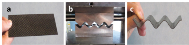
Fig. 3 Thermoforming of a cured composite laminate. A 2 mm thick carbon fibre reinforced dynamic epoxy laminate (a) was compression-moulded in a zig-zag shaped mould (b), rendering a thermoformed wavy 3D part (c). Reproduced with permission from ref. 43. Copyright 2016 Royal Society of Chemistry.
