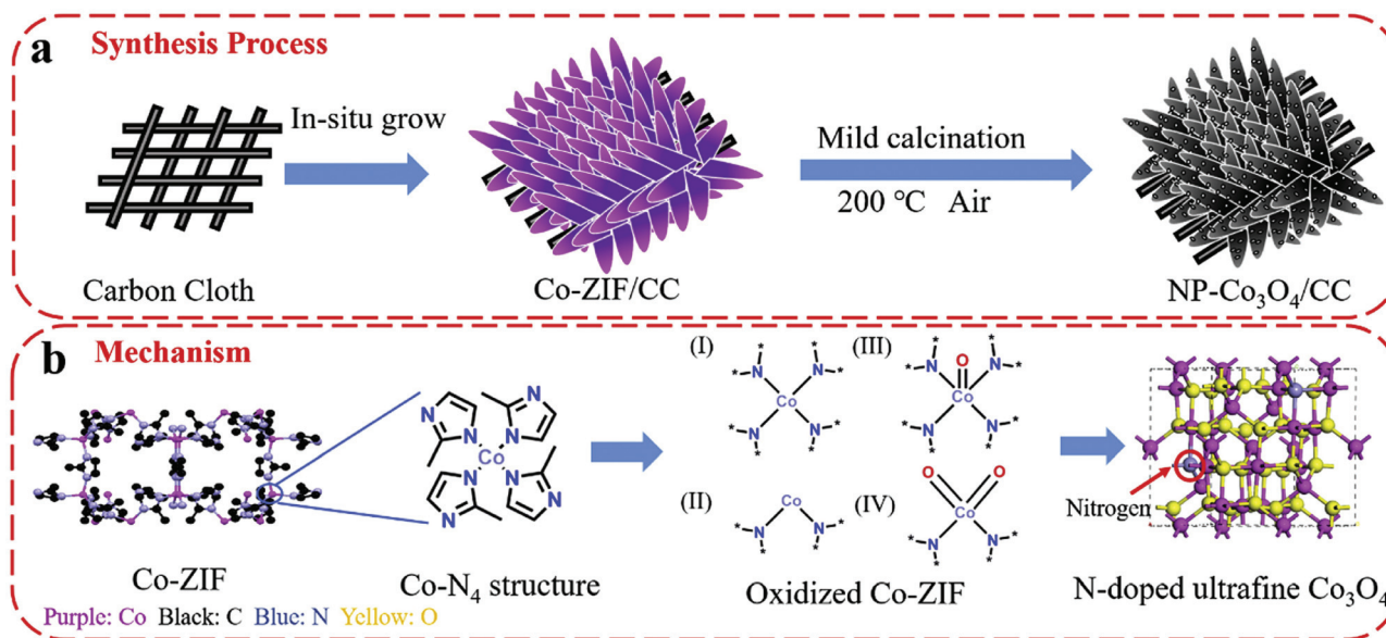
Fig. 14 Schematic demonstration of (a) the fabrication process of NP- \text{Co}_3\text{O}_4/\text{CC} and (b) the proposed mechanism of nitrogen doping in cobalt oxide lattices. Reproduced from ref. 282 with permission from Elsevier B.V.
