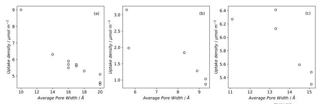
Fig. 1 Uptake densities of (a)  $H_2$  at 1 bar and -196 °C, (b)  $CO_2$  at 1 bar and 25 °C, and (c)  $CH_4$  at 65 bar and 25 °C on carbons<sup>79,194,219</sup> as a function of average pore size.
