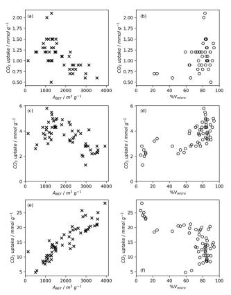
Fig. 3 Trends in BET surface area and percentage micropore volume with CO<sub>2</sub> uptake capacity of carbons 78,80,81,135,237,238,244,248 at 0.15 bar (a) and (b), 1 bar (c) and (d), and 20 bar (e) and (f).
