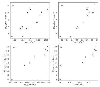
Fig. 4 Trends in CH<sub>4</sub> uptake with gravimetric (a) and (b) and volumetric (c) and (d) porosity of carbons  $^{35,131,258}$  at 35 bar and 25 °C.
