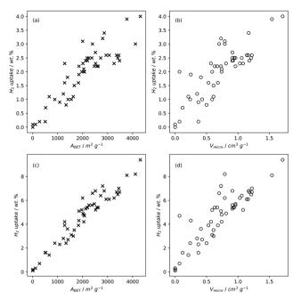
Fig. 2  $\rm H_2$  uptake of carbons at  $-196~^{\circ}$ C and 1 bar (a) and (b) or 20 bar (c) and (d) as a function of BET surface area (a) and (c) or micropore volume (b) and (d).  $^{79,82,83,196,220,221}$
