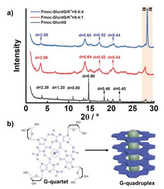
Fig. 5 (a) XRD patterns of hydrogels of Fmoc-Glu/dG, Fmoc-Glu/dG/K<sup>+</sup> (8:4:1, molar ratio) and Fmoc-Glu/dG/K+ (8:4:4, molar ratio). (b) Formation and stacking of G-quartets
