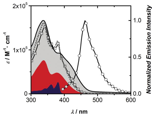
Fig. 3 Molar absorption coefficients in DCM of **1** (squares,  $10^{-5}$  M) and its fluorescence spectrum (excitation 381 nm, circles) compared to building blocks PTZ **2** (red fill) and NDI **3** (blue fill) in DCM. The grey dashed line represents the addition of **2** and **3** in a 2:1 summative ratio and the black line (grey fill) represents the normalized solid-state film absorption profile of **1**.
