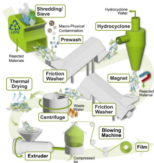
Fig. 15 Mechanical recycling process of polyethylene plastic film at an industrial plant. 175
