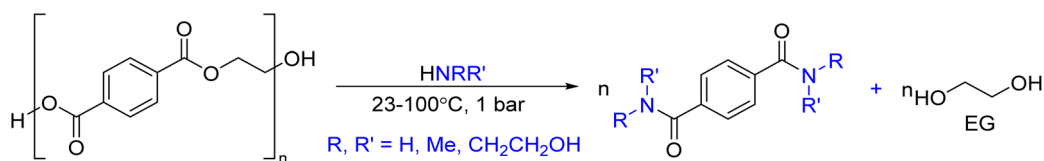
Fig. 34 Typical reaction conditions and products for PET aminolysis.
