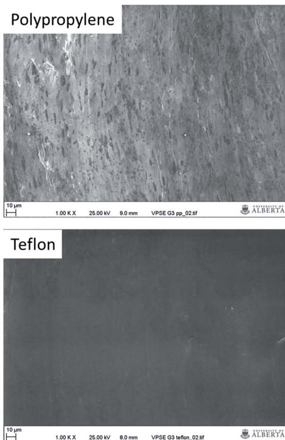
Fig. 5 Scanning electron microscopy images of unused polypropylene (PP) and Teflon. Black spots on the PP represent a porous surface.
