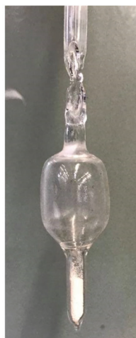
Fig. 1 Diagram and actual picture of a quartz cell used for measuring Raman spectra under static equilibrium. The cell is sealed under \text{O}_2(\text{g}) , p_{\text{O}_2} = 0.19 atm.
