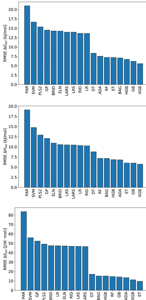
Fig. 1 Root-mean-squared error (RMSE) of predicted  $\Delta G_{\text{sol}}$  (top panel),  $\Delta H_{\text{sol}}$  (middle panel) and  $\Delta S_{\text{sol}}$  (bottom panel) after a leave-one-out (LOO) permutation approach for each data point in accordance with different machine learning methods.
