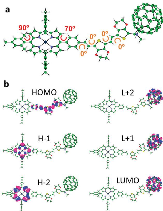
Fig. 1 (a) Minimum-energy structure (characteristic dihedral angles are indicated) and (b) frontier molecular orbital contours (isovalue =  $\pm 0.03$ ) calculated for triad **1** at the B3LYP/cc-pVDZ+LANL2DZ(Zn) level including solvent effects. H and L denote HOMO and LUMO, respectively.
