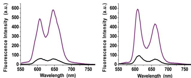
Fig. 6 Steady-state fluorescence spectra of **ZnP** (purple line) and **ZnP-2EDOTV-C<sub>60</sub>** (**1**, black line) in toluene (left) and benzonitrile (right).  $\lambda_{exc} = 426$  nm. Concentration  $10^{-6}$  M.
