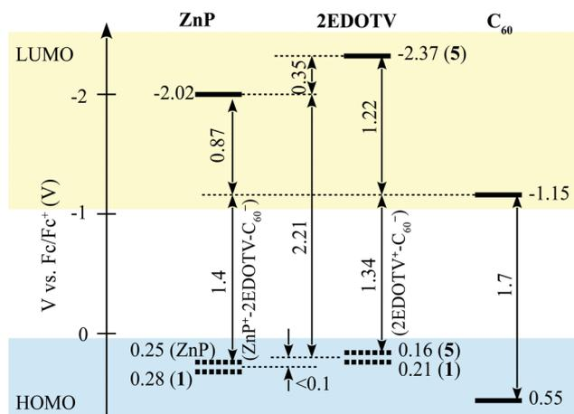
Fig. 2 Relative energy positions of HOMO and LUMO levels of the chromophores constituting the Zn-2EDOTV- $C_{60}$  triad.
