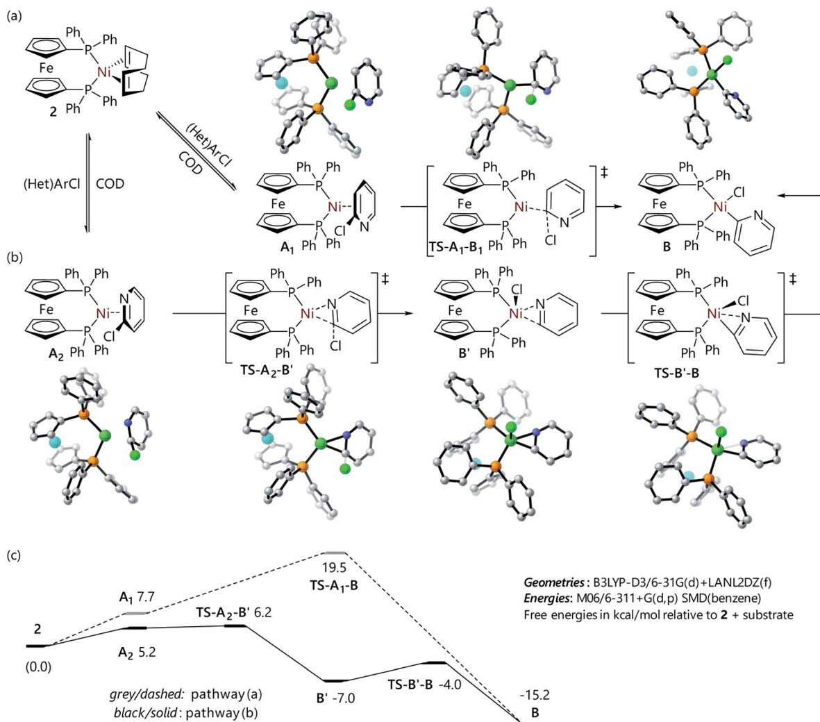
Fig. 3 Structures for the reaction of 2-chloropyridine with **2** via (a) an  $\eta^2(\text{C}=\text{C})$  complex and (b) an  $\eta^2(\text{C}=\text{N})$  complex, and (c) free energy profiles for these reactions.
