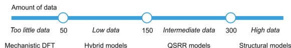
Fig. 13 Models for quantitative rate prediction for different data regimes based on the S_NAr dataset.
