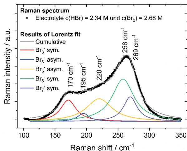
Fig. 8 Raman spectrum of the electrolyte mixture with  $c(\text{HBr}) = 2.34 \text{ M}$  and  $c(\text{Br}_2) = 2.68 \text{ M}$  (SOC = 80%) and water including Raman fitting for the symmetrical and antisymmetrical stretching oscillation of tribromide, pentabromide and heptabromide.
