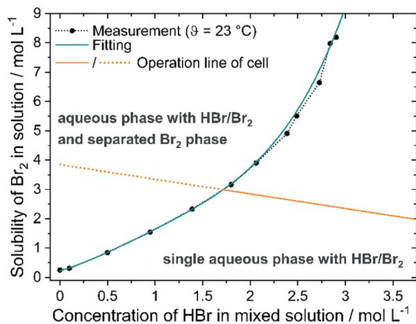
Fig. 5 Solubility of Br<sub>2</sub>  $c(\text{Br}_2)_{\text{sat}}$  in aqueous HBr solutions  $c(\text{HBr})_{\text{sat}}$  as a function of the HBr concentration in the solution (black dots and green fitting line) and superposition with the operation line (orange line) of the H<sub>2</sub>/Br<sub>2</sub>-RFB electrolyte by stoichiometric concentration change.
