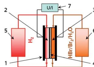
Fig. 1 Principle of a H<sub>2</sub>/Br<sub>2</sub> redox flow battery with (1) energy converter including (2) H<sub>2</sub> negative half cell, (3) Br<sub>2</sub>/Br<sup>-</sup> positive half cell and (4) membrane in the middle and media storage tanks for (5) H<sub>2</sub> and (6) HBr/Br<sub>2</sub>/H<sub>2</sub>O electrolyte on left and right side and (7) grid connection.
