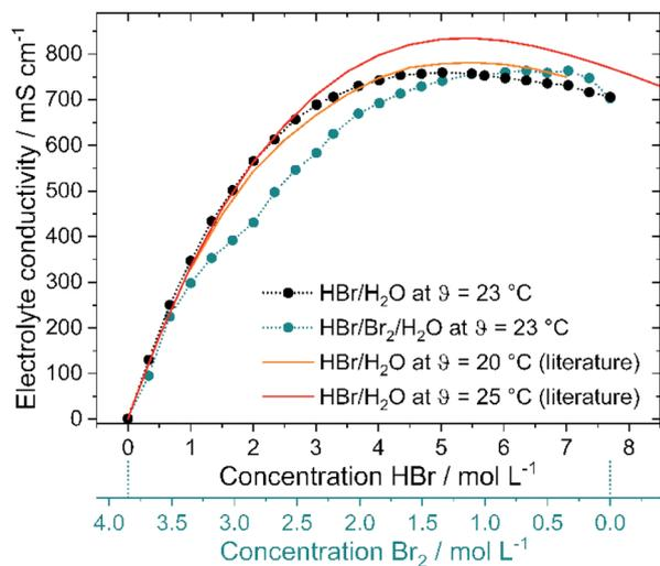
Fig. 6 (a) Electrolyte conductivities as a function of the concentration of HBr  $c(\text{HBr})$  in a pure HBr solution and HBr/Br<sub>2</sub> solution for a bromine half cell. Measurements shown as points and literature values as lines [11,53] and (b) quantitative ratio between water H<sub>2</sub>O and HBr in the investigated electrolyte solutions as a function of the HBr concentration.
