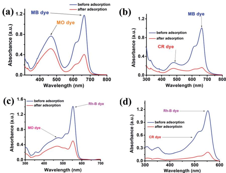
Fig. 8 Adsorption plots of MB (a and b) and Rh-B (c and d) in the presence of MO and CR using the {Fe<sub>3</sub>} cluster as the adsorbent.
