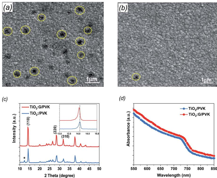
Fig. 3 (a) FESEM image of perovskite deposited on a pure  $TiO_2$  layer. (b) Perovskite on a G: $TiO_2$  layer. (c) XRD patterns of perovskites. The asterisk indicates the reflection of  $PbI_2$ . Inset: zoomed-in view of the peak at 14° of the perovskites. (d) Absorption spectra of perovskite films deposited on pure and modified  $TiO_2$  layers.
