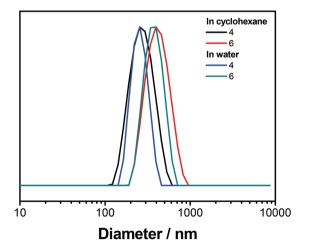
**Fig. 4** Diameters of PU-nanocarriers containing either monomer **4** or **6**. The measurement was performed in cyclohexane (black, red) or after transferring to water in an aqueous solution (blue, green).
