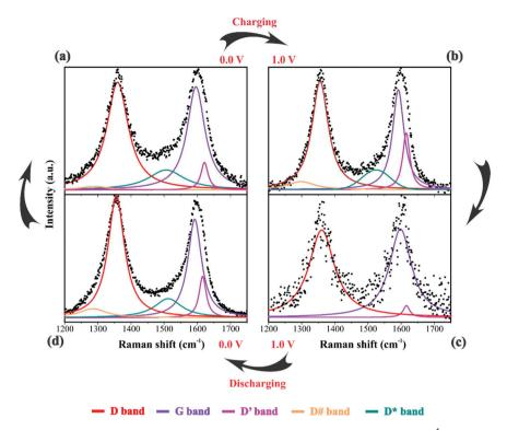
Fig. 6 Raman spectra of the electrode/electrolyte interface under cyclic voltammetry at scan rate 0.15 mV s<sup>-1</sup> from (a) 0 V to (b) 1 V during charge and from (c) 1 V to (d) 0 V during discharge. Spectra intensities are normalized from 0 to 1 in the 1200 to 1750 cm<sup>-1</sup>. Electrodes were housed in an El Cell filled with 80  $\mu$ L of a 1 M Li<sub>2</sub>SO<sub>4</sub> aqueous solution. Deconvolution considered five bands as described in Fig. 1(d).
