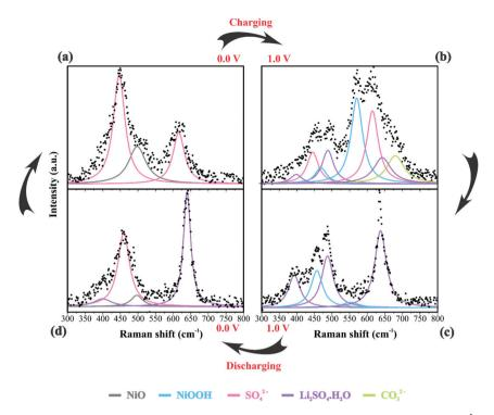
Fig. 4 Raman spectra of the electrode/electrolyte interface under cyclic voltammetry at a scan rate of 0.15 mV  $\rm s^{-1}$  from (a) 0 to (b) 1 V during charge and from (c) 1 V to (d) 0 V during discharge. Spectra intensities are normalized from 0 to 1 in the 300 to 800 cm<sup>-1</sup>. Working electrodes were housed in a symmetrical El Cell filled with 80 µL of a 1 M Li<sub>2</sub>SO<sub>4</sub> aqueous solution.
