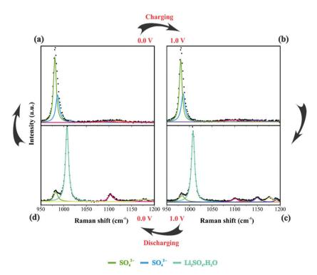
Fig. 5 Raman spectra of the electrode/electrolyte interface under cyclic voltammetry at scan rate 0.15 mV s<sup>-1</sup> from (a) 0 V to (b) 1 V during charge and from (c) 1 V to (d) 0 V during discharge. Spectra intensities are normalized from 0 to 1 in the 950 to 1200 cm<sup>-1</sup>. Electrodes were housed in an El Cell filled with 80  $\mu L$  of a 1.0 M Li<sub>2</sub>SO<sub>4</sub> aqueous solution.
