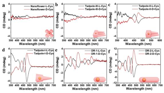
Fig. 10 (a-f) Mirror symmetry CD spectra of the L-/D-CdSe/CdS NCs having different shapes such as (a) nanoflowers, (b) Tadpole-III, (c) Tadpole-II, (d) Tadpole-I, (e) short dot/rods, and (f) long dot/rods. Reprinted with permission. 91 Copyright 2020, American Chemical Society,
