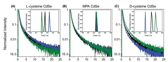
Fig. 16 (A-C) Lifetime decay profiles for acceptor CdSe QD functionalized with chiral L-cysteine, achiral mercaptopropionic acid, and chiral D-cysteine, respectively. Data represented in black, blue, and green correspond to the linear, clockwise, and counter-clockwise circularly polarized excitation light, respectively. Insets show the short parts of the lifetime distributions. Reprinted with permission. 108 Copyright 2017, American Chemical Society.
