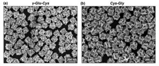
Fig. 7 (a) SEM images reveal crystal facets of chiral Au NPs generated by  $\gamma$ -Glu-Cys, and (b) Cys-Gly, respectively. Reprinted with permission. Reprinted with permission. Copyright 2020, Wiley-VCH.
