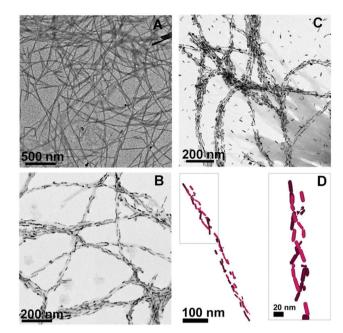
Fig. 19 TEM images of (A)  $\alpha$ -synuclein fibrils, (B)  $\alpha$ -synuclein fibrils mixed with 0.5 nM Au NRs, (C) 2.0 nM Au NRs, and (D) 3D chiral structure of Au NRs. Reprinted with permission.<sup>131</sup> Copyright 2018, the National Academy of Sciences of the United States of America.
