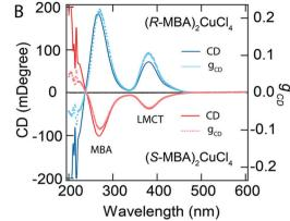
Fig. 12 (A) UV-vis-NIR spectra, and (B) CD spectra with the corresponding anisotropy factors of (R-/S-/rac-MBA)<sub>2</sub>CuCl<sub>4</sub> and (PEA)<sub>2</sub>CuCl<sub>4</sub>. Optical images of (PEA)<sub>2</sub>CuCl<sub>4</sub> and (R-MBA)<sub>2</sub>CuCl<sub>4</sub> crystals are shown in the inset. Reprinted with permission. 104 Copyright 2021, American Chemical Society.
