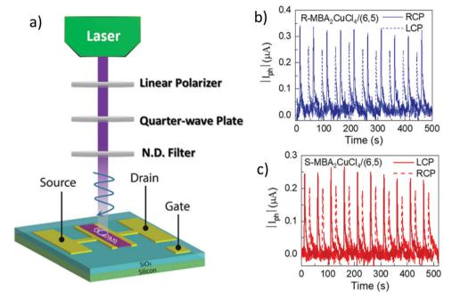
Fig. 14 (a) Schematic description of an experimental set-up used for creating left and right CPL. (b) Photocurrent (μA) variation as a function of time (s) using R-MBA<sub>2</sub>CuCl<sub>4</sub>/SWCNT, and (c) S-MBA<sub>2</sub>CuCl<sub>4</sub>/SWCNT when illuminated with a 405 nm pulsed laser light under  $V_{DS} = 2$  V. Reprinted with permission.<sup>104</sup> Copyright 2021, American Chemical Society.
