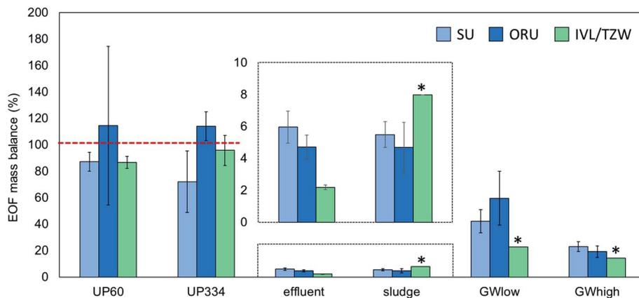
Fig. 2 EOF mass balance (%) in interlaboratory comparison samples. Error bars represent pooled standard deviation ( $n = 3$  for EOF and  $\sum$ PFAS-16). The dashed red lines indicate the expected EOF mass balance. \* indicates that only a single measurement was performed.
