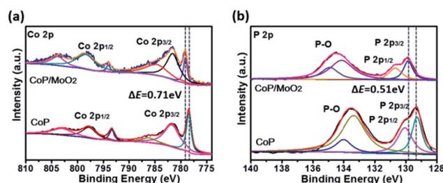
Fig. 1 XPS spectra of porous CoP/MoO<sub>2</sub> thin films and pure CoP thin films: (a) Co 2p spectra, (b) P 2p spectra.
