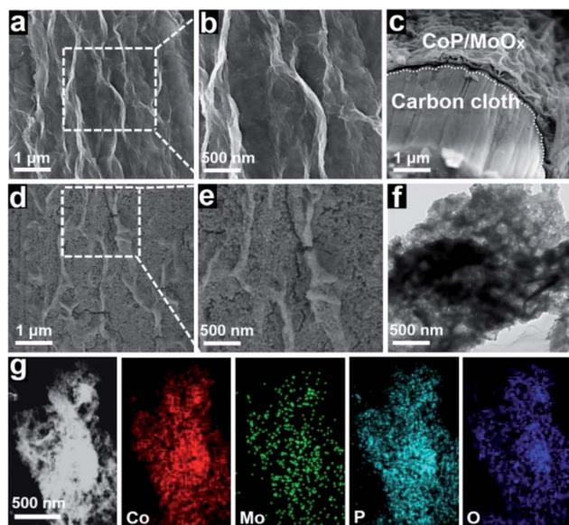
Fig. 2 (a and b) SEM image and magnified SEM image of CoP/MoO<sub>x</sub> thin films. (c) SEM image of the cut surface of CoP/MoO<sub>x</sub> thin films. (d and e) SEM images of porous CoP/MoO<sub>2</sub> thin films. (f) TEM image of a typical porous CoP/MoO<sub>2</sub> thin film. (g) HAADF-STEM image and elemental mapping images of Co, Mo, P and O in the porous CoP/MoO<sub>2</sub> thin films.
