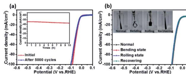
Fig. 4 (a) Accelerated durability test on the porous CoP/MoO<sub>2</sub> thin film electrode. (b) Polarization curves of the porous CoP/MoO<sub>2</sub>-CC electrode under different distortions. Inset images in (b) are the optical photographs of the working electrode at different testing states.
