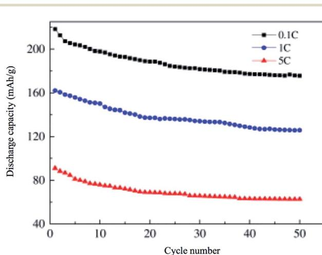
Fig. 17 Cyclic performance of nano  $\text{C}/\text{Li}_2\text{MnSiO}_4$  synthesized by ionothermal method, the material is tested in the potential range of  $2.5\text{--}4.5 \text{ V}$ .<sup>153</sup>
