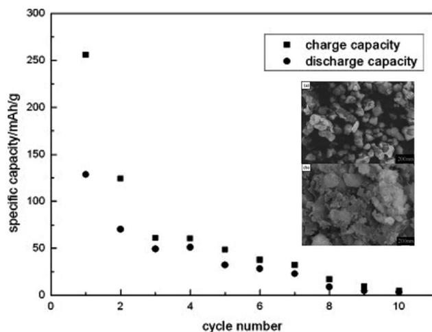
Fig. 16 Cyclic performance of  $\text{Li}_2\text{MnSiO}_4$  synthesized by solid state method tested at  $C/16$  rate to a cut-off voltage between  $1.5$  and  $4.8 \text{ V}$ .<sup>152</sup> The inset shows FESEM micrographs of (a)  $\text{Li}_2\text{MnSiO}_4$  and (b)  $\text{Li}_2\text{MnSiO}_4/\text{C}$ .
