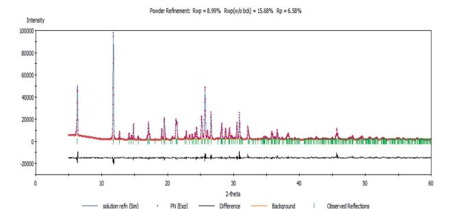
Fig. 1 The Rietveld refinement plot showing an agreement between the calculated and measured X-ray powder diffractograms of the complex.
