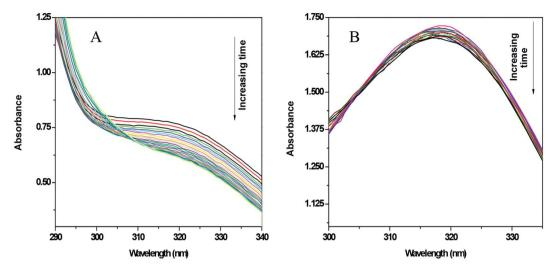
Fig. 6 UV-vis spectra of Onz (A) and  $Zn(Onz)_2Cl_2$  (B) in the presence of hypoxanthine in 5% DMF and xanthine oxidase. Spectra of each compound were taken at intervals of 5 minutes for 2 hours. Enzyme activity = 0.2 units per mL in XOD and compound concentration = 80  $\mu$ M.
