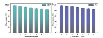
Fig. 8 CS/GA/RGO/Pd composite hydrogel catalyzes the stability of 4-NP (a) and 2-NA (b) in different continuous cycles.
