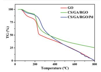
Fig. 4 TG curves of GO, CS/GA/RGO hydrogel, CS/GA/RGO/Pd hydrogel.
