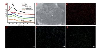
Fig. 3 XRD patterns (a) of CS, GO, CS/GA/GO hydrogel, CS/GA/RGO hydrogel, CS/GA/RGO/Pd hydrogel; SEM image (b) and element mappings (c-f) of CS/GA/RGO/Pd hydrogel.
