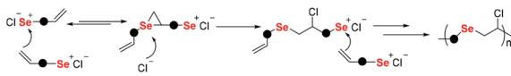
Scheme 5 The novel addition reaction of electrophilic selenium reagents and sulfonyl chloride. Reproduced with permission from ref. 54. Copyright 2019 The Royal Society of Chemistry.
