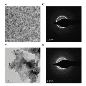
Fig. 4 (a) EM micrograph of 1 mg mL $^{-1}$  P3. (b) EM diffraction pattern of 1 mg mL $^{-1}$  P3. (c) Transmission electron microscopy image of 1 mg mL $^{-1}$  P3. (b) Transmission electron microscopy diffraction pattern of 1 mg mL $^{-1}$  P4.
