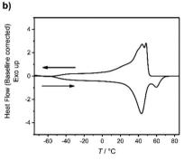
Fig. 3 (a) Transmission electron microscope micrograph of the single P3 crystals (0.1 mg mL $^{-1}$ ). (b) Differential scanning calorimetry (baseline corrected) of P3 showing the second heating and cooling curve with a  $T_{\rm q}$  at -49 °C and  $T_{\rm m}$  at 58 °C determined in the second heating curve.
