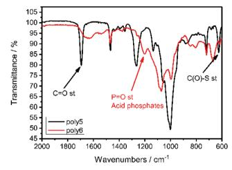
Fig. 5 FTIR spectrum of P3 and P4 (after two step reaction) highlighting the important frequencies.
