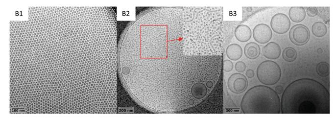
Fig. 7 Representative cryo-TEM images of the crude latexes B1-B3 (Table 1).
